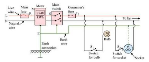
• **Switches**: It is a device which is connected in the live wire so as to turn 'ON' or 'OFF' the current in the circuit.
